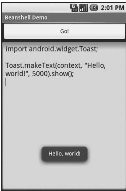
Figure 21-2. The AndShell BeanShell IDE, executing some code
